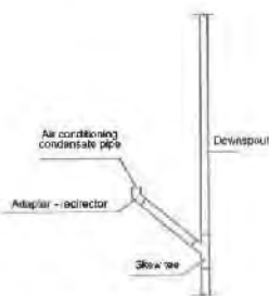
The node of air condition drain
