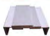
0.7mm HPL+4mm Plywood +12mm Fir Wood +0.7mm HPL;
